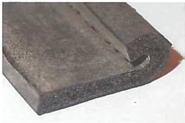
Photo 19: This is a close-up of the original gearbox cover seal. The material is mold- ed, skinned foam rubber approximately 1/8 inch thick. Measured from the top of the curve, the long leg is 7/8 inch and the short one about 1/4 inch.
